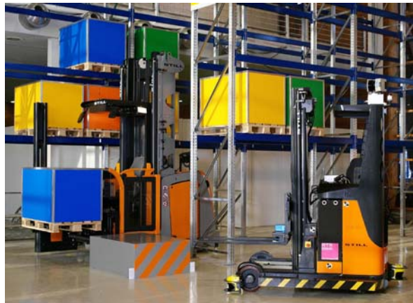
Figure 6. RTS-STILL Robotic Fork-Lift, as presented at the CeMAT 2005
