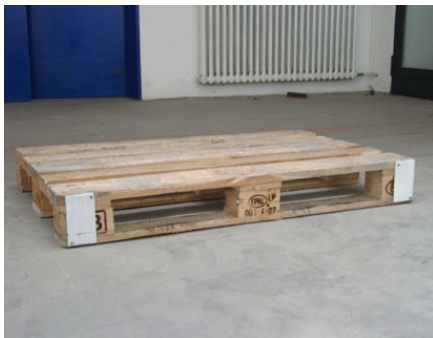
Figure 2. Palette modified with reflectors
