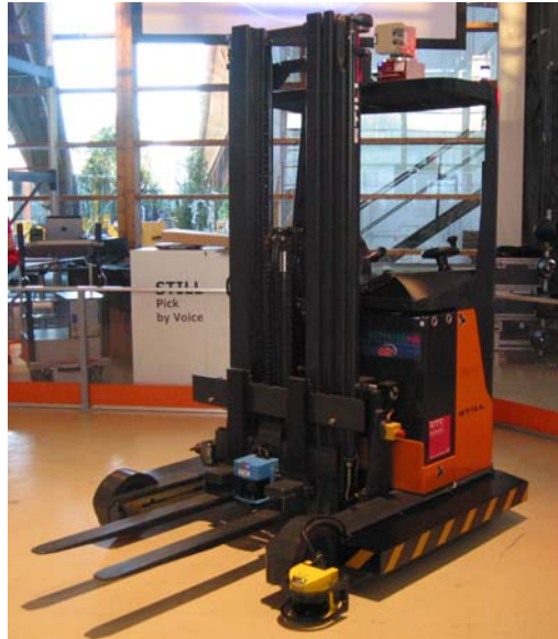
Figure 1. The project platform: Still FM14i with additional sensors for autonomous operation.
