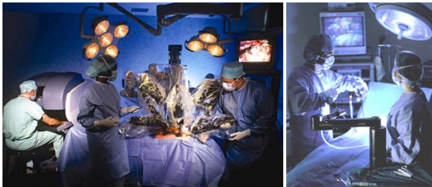
Figure 15: Commercially available surgical robots (left) daVinci (Intuitive Surgical Inc.), (right) AESOP (Computer Motion Inc.)
