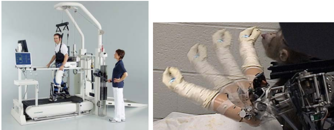
Figure 14: Rehabilitation robotics (left) LokoMat (Hocoma AG, Switzerland); (right) prosthetic arm controlled by the monkeys brain signals (University of Pittsburgh)
