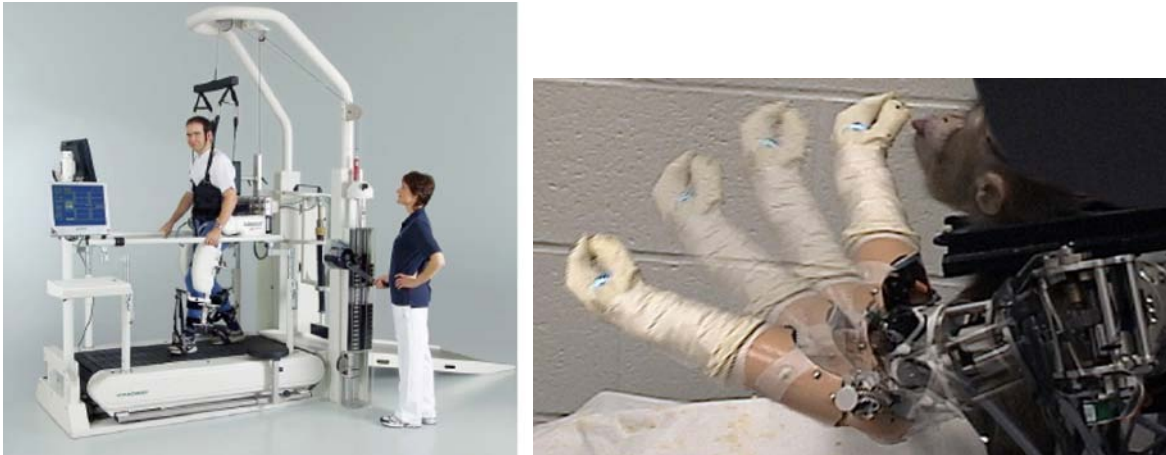
Figure 14: Rehabilitation robotics (left) LocoMat (Hocoma AG, Switzerland); (right) prosthetic arm controlled by the monkeys brain signals (University of Pittsburgh)
